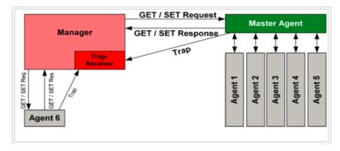
An SNMP trap port is the port at which the manager receives the traps. This port is typically set as port number 162. However, you can change this port if necessary, and it may also differ depending on the SNMP manager you're using.
